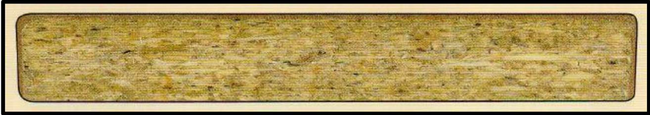
**Moisture Resistant Particle Board (PB)** is perfect for use in places with high humidity levels. In comparison to standard PB, Moisture Resistant PB contains a moisture-repellent resin which gives it a better moisture resistant rating. However, moisture resistant PB shouldn't be mistaken to be 100 percent water resistant as it's still prone to swelling and warping if in direct contact with such elements.
